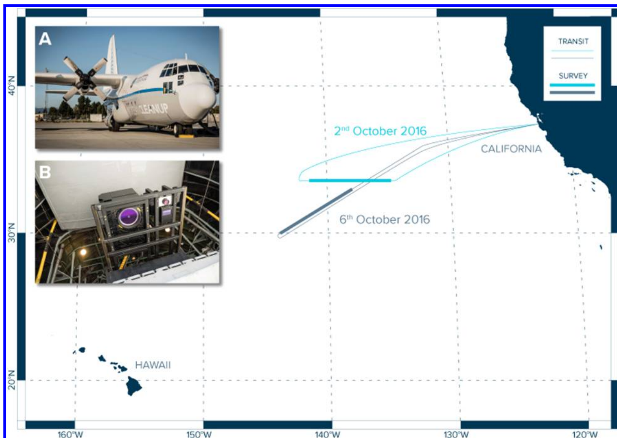
Figure 1. Map showing the area surveyed on October 2 (light blue track) and October 6 (dark blue track) 2016. While in survey mode (thicker lines), the sea surface area below the aircraft was imaged with a SWIR imager and a RGB camera. (A) Image of the Lockheed C-130 Hercules aircraft used in this study. (B) Customized frame used to attach the SASI imager and the RGB camera to the rear ramp of the aircraft, at nadir position. We also surveyed the area with a bathymetric lidar, but the results are not described in this study.
