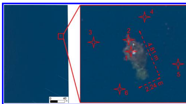
Figure 4. RGB image of the ghost net used for most of the analyses described in this study. Red stars show regions where spectral information from the SWIR imagery were extracted: “floating part” (star 1), “submerged part” (star 2), and “seawater” (stars 3–6).
